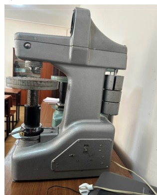
Figure 4. Devices used to determine the microhardness and hardness of parts ("ПМТ-3М" - a, "TKC - 1M" and "Buehler" - b).
