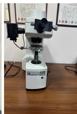
Figure 4. Devices used to determine the microhardness and hardness of parts ("ПМТ-3М" - a, "TKC - 1M" and "Buehler" - b).
