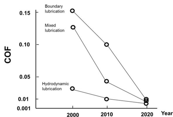
*Fig. 2. The development of lubricants has reduced friction in different lubrication regimes, and this trend will continue in the near future (modified from Holmberg, 2012).*
