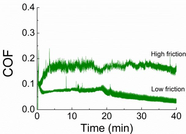
Fig. 6. Two friction curves measured in a stainless steel vs stainless steel POD experiment. Although the conditions were identical, the friction was significantly lower in the second experiment. The contacts were lubricated with FpHYD5 in 50 mM acetate buffer. The test parameters were normal load 10 N, sliding velocity 0.1 m/s and duration 40 min.
