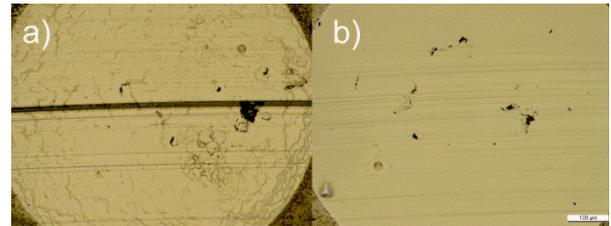
Fig. 7. a) Tribofilm formed on the stainless steel surface, b) no tribofilm formed.
