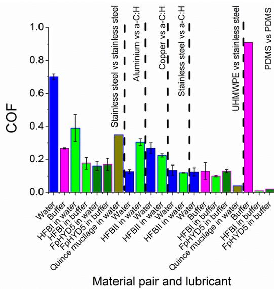
Fig. 5. Lubrication of different material pairs with water, 50 mM sodium acetate buffer, hydrophobin proteins and quince mucilage. (Publications I-VI; Hakala and Lee, 2011)
