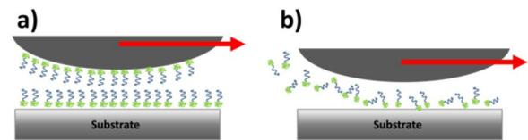
Fig.8. a) A situation in which hydration lubrication is possible in a POD experiment, b) a situation with hard materials in which wear and shear force have removed molecules from the upper surface, which is constantly in contact.
