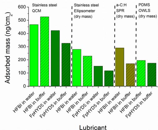
Fig. 4. Adsorbed mass of hydrophobins on different surfaces. Ellipsometer, SPR and OWLS measure the dry mass of hydrophobins adsorbed on the surface while QCM takes bound water into account (Publications II and V; Hakala and Lee, 2011).
