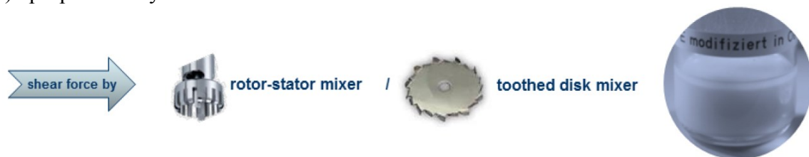
Scheme 1. Oil-PTFE-cc dispersion (PTFE up to 25 wt-% = liquid).
