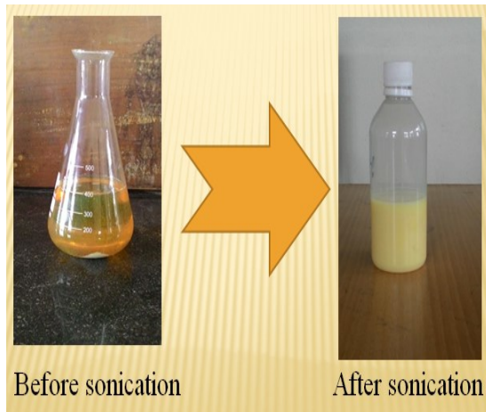
Figure 1. Ultrasonic cleaner and lubricant before and after sonication
