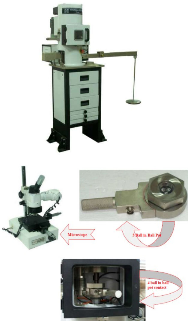
Figure 2. Four-ball tester machine and its various parts
