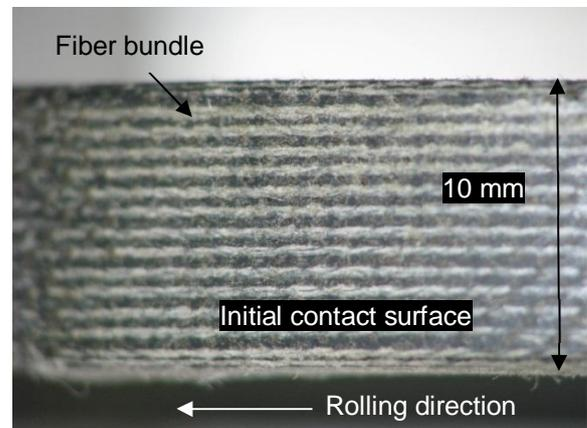
Figure 2. Photomicrograph of the initial contact surface of polymer composite.
