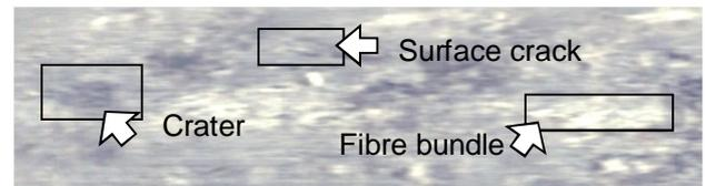
Figure 5. Stitched image after 2 hours of testing.
