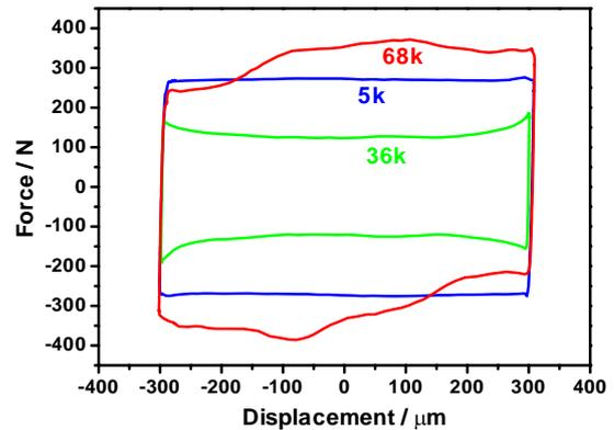
Figure 5. Fretting loops obtained from EMV rig for 5k, 36k and 68k.
