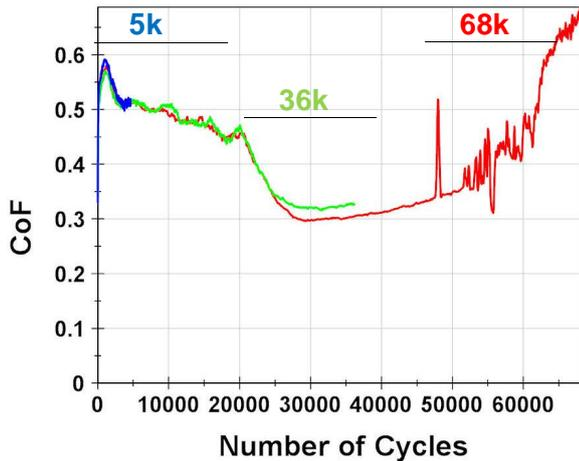
Figure 4. Evolution of coefficient of friction with fretting cycles. Three tests conducted under identical conditions are included, with tests being terminated at different points.
