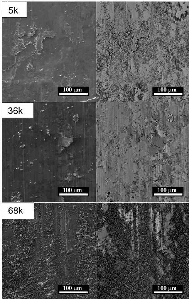
Figure 7. SE (left) and BSE (right) plan view micrographs of representative portions of the wear scars at 5k, 36k and 68k cycles.
