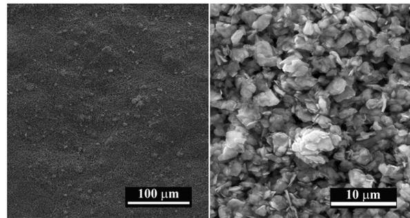
Figure 2. Low magnification (left) and high magnification (right) SEM micrograph of the surface of the as-cured DFL paint coating MoS<sub>2</sub>.
