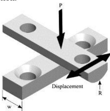
Figure 1. Cylinder-on-flat specimen setup for the fretting test [13], where  $w = 10 \text{ mm}$ ,  $R = 15 \text{ mm}$  and  $P = 575 \text{ N}$ .
