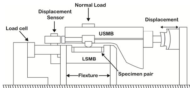
Figure 3. A schematic diagram of the fretting rig.
