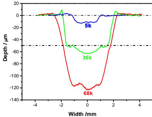
Figure 6. Average profiles of the wear scar after 5k, 36k and 68k cycles. The dotted lines indicate the location of the DFL coating.
