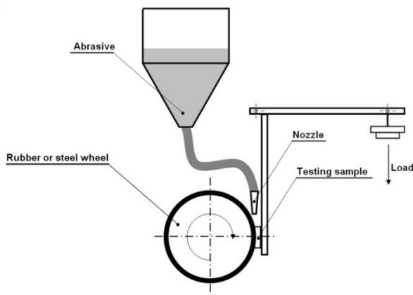
Figure 2. Schematic diagram of the ASTM G65 abrasion test rig.
