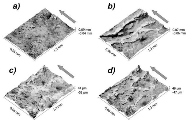
Figure 6. 3D surface topography within the wear scar generated during the tests with the rubber wheel for: a) Polymer A; b) Polymer B; c) Polymer C; d) Polymer D
