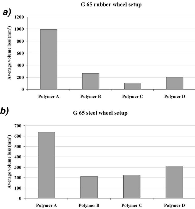
Figure 3. Average volume loss for the selected polymer materials in the 1.5 hr experiments: a) ASTM G65 rubber wheel setup; b) ASTM G65 steel wheel setup
