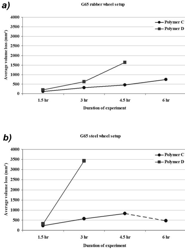
Figure 5. Average volume loss for selected polymer materials after the 6 hr experiments: a) ASTM G65 rubber wheel setup; b) ASTM G65 steel wheel setup.
