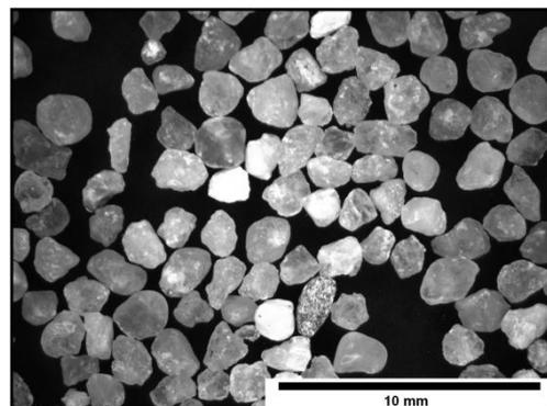
*Figure 1. Abrasive particles used in the experiments (Image of abrasive particles before experiment).*
