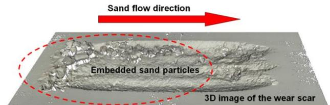
Figure 8. 3D surface topography of Polymer C wear scar from a 6 hours experiment (The arrow shows the direction of motion of the wheel surface, and the main direction of the abrasive sand).
