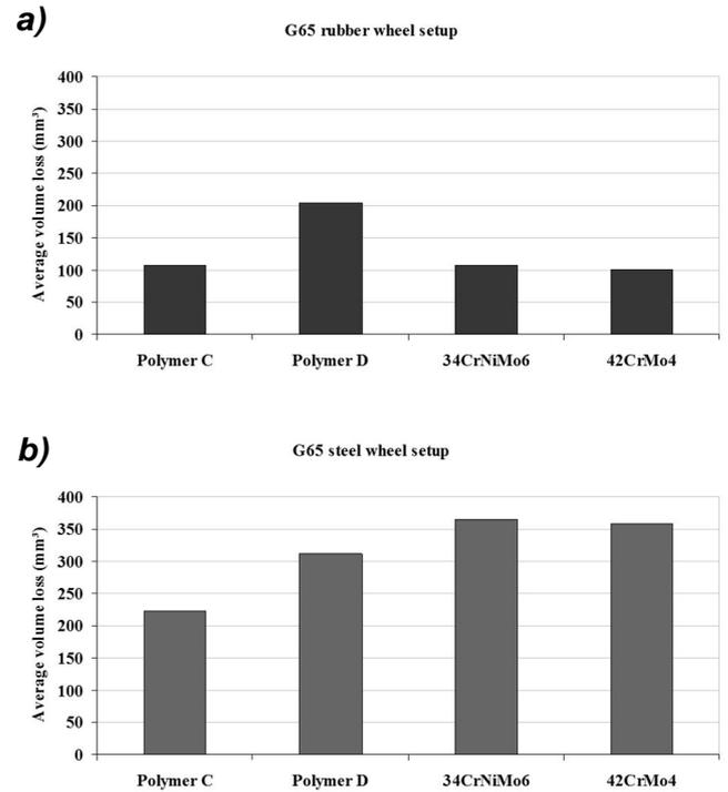
Figure 4: Average volume loss of best performing polymers and selected steel materials.
