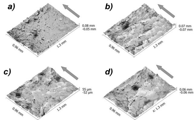
Figure 7. 3D surface topography within the wear scar generated during the tests with the steel wheel for: a) Polymer A; b) Polymer B; c) Polymer C; d) Polymer D
