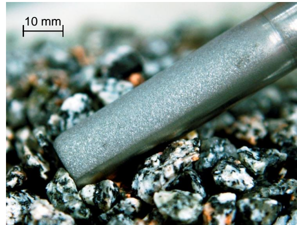
Figure 3. Round AISI 316 sample with granite gravel.
