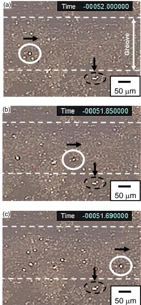
Figure 8. Results of in situ observations in the case of Type 2 pin: (a) 0.00 s, (b) 0.15 s, and (c) 0.31 s.
