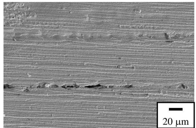
Figure 12. SEM images of wear tracks on the textured surface in the case of Medium.
