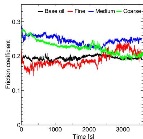
Figure 1. Variation in friction coefficient behavior as a function of sliding time.
