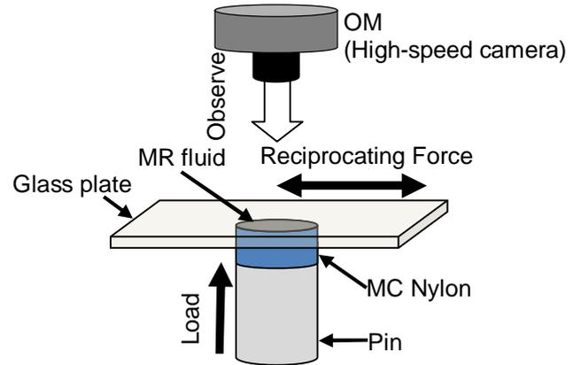
Figure 5. Schematic of device used for *in situ* observations.
