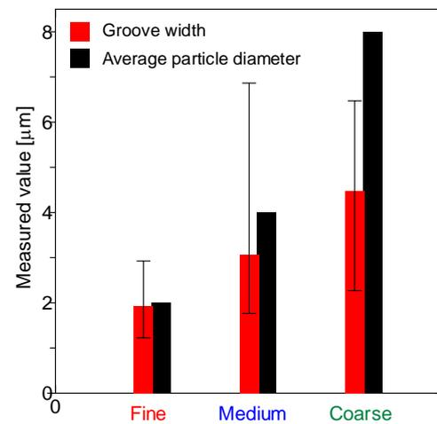
Figure 9. Relationship between FM particle diameter and groove width.
