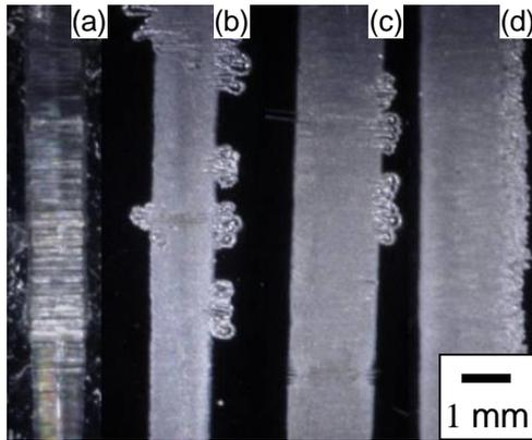
Figure 2. OM images of wear tracks: (a) Base oil (b) Fine (c) Medium, and (d) Coarse.
