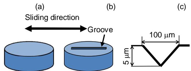
Figure 6. Pins used: (a) Type 1 and (b) Type 2. (c) Shape of groove.
