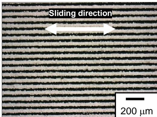
Figure 10. Surface texture of the disk specimens.
