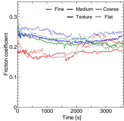
Figure 11. Variation in friction coefficient behavior as a function of sliding time in the case of the textured surface.
