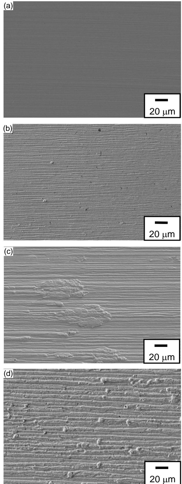
Figure 4. FE-SEM images of wear tracks: (a) Base oil (b) Fine (c) Medium, and (d) Coarse.
