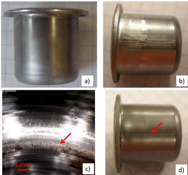
Figure 9: Specimen results a) EN 1.4301; b) DP 800 with severe galling; c) pick-up on V4E die 3 tested with DP 800; d) DP 800 with no significant galling (the arrow indicates local, light galling).
