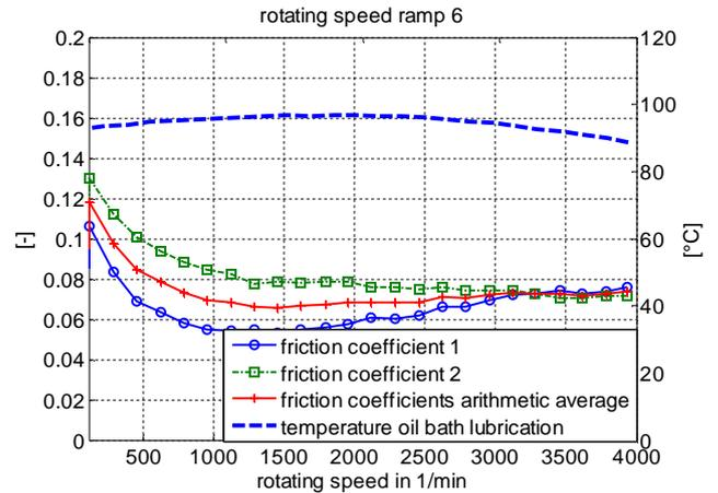
Figure 10. Friction coefficients and temperature of the oil bath lubrication at rotating speed ramp 6.
