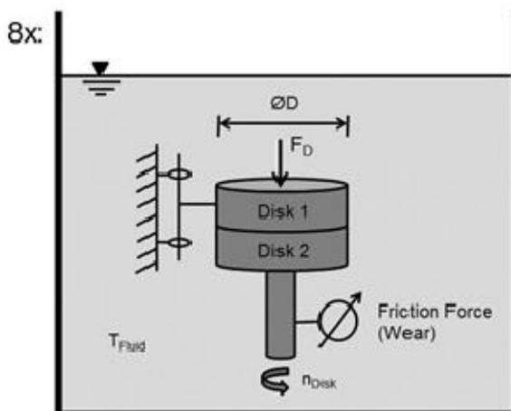
Figure 2. Modeling of the test bench RPR.
