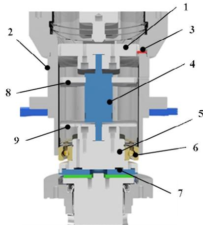
Figure 4. Torque damper for the non-rotating test components with friction force measurement system.
