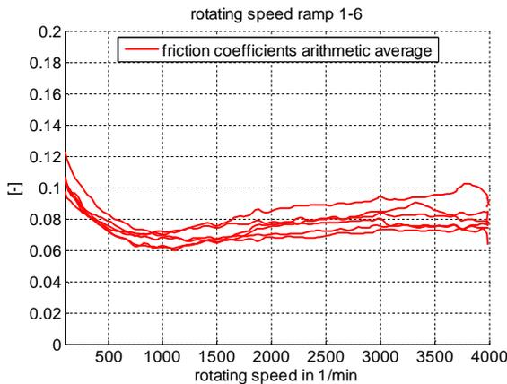
Figure 11. Arithmetic averages of the measured friction coefficients at rotating speed ramp 1 to 6.
