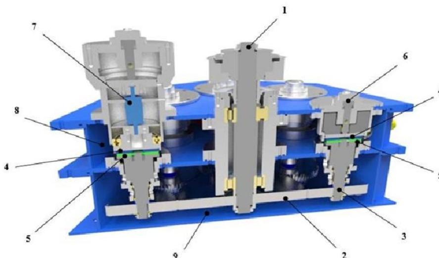
Figure 5. Sectional view test chamber test bench RPR.
