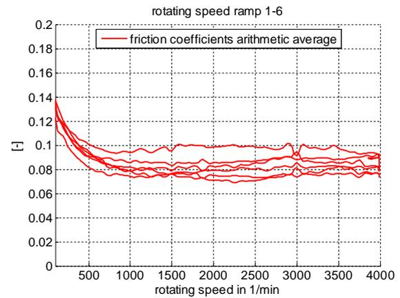
Figure 12. Arithmetic averages of the measured friction coefficients at rotating speed ramp 1 to 6 with changed test components at the friction force measurement mounts.
