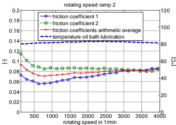
Figure 9. Friction coefficients and temperature of the oil bath lubrication at rotating speed ramp 2.
