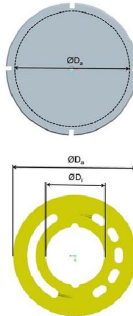
Figure 6. Geometry of the nonrotating disk (left) and rotating disk (right).
