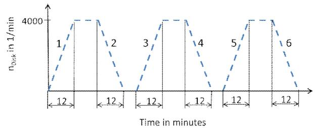
Figure 7. Validation test procedure for the test bench RPR.
