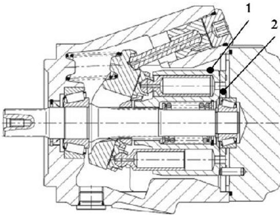
Figure 1. Axial piston variable pump, design Bosch-Rexroth, type A10VNO [1].
