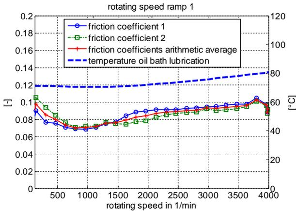
Figure 8. Friction coefficients and temperature of the oil bath lubrication at rotating speed ramp 1.
