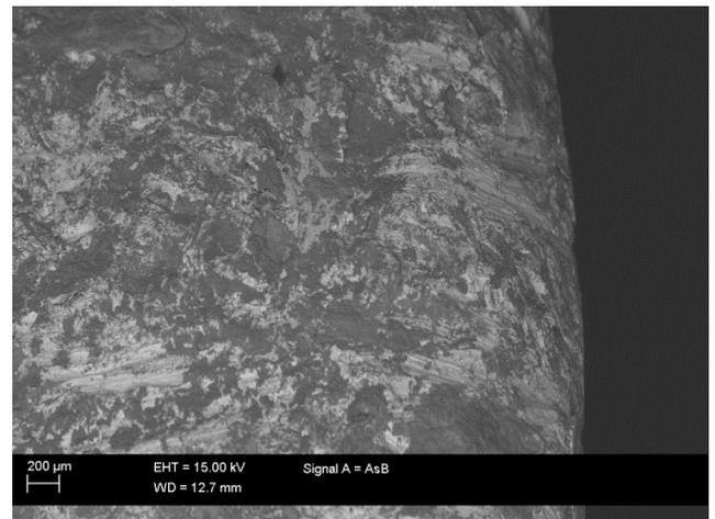
Figure 4. Worn outer edge of the S355 outer pin after the test. Specimen is tilted 45° with respect to the wear surface normal.
