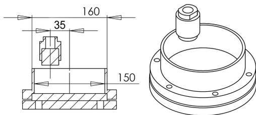
Figure 1. Schematic of the crushing pin-on-disk test device.
