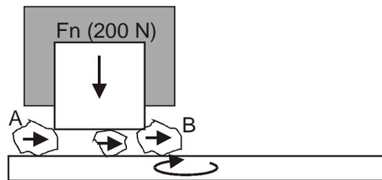
Figure 2. Illustration of the interaction between large rocks and the specimen edges in the crushing pin-on-disk test. The specimen holder is colored dark grey.
