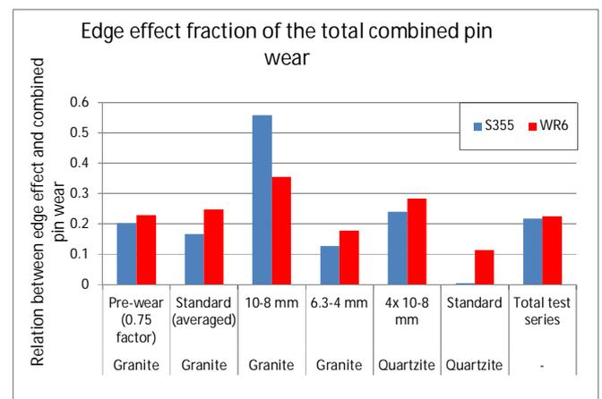
Figure 12. Edge effect fraction of the combined pin wear in different tests, including the total wear of the entire test series.
