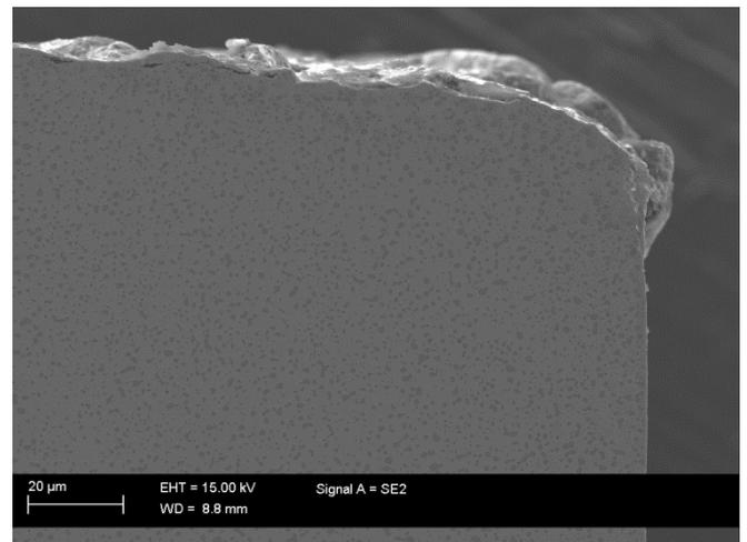
Figure 10. Cross-section of the edge of the WR6 inner pin. The edge radius is about 20 µm.
