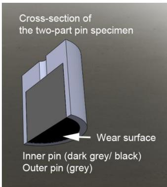
Figure 3. Cross-section of the two-part pin specimen.
