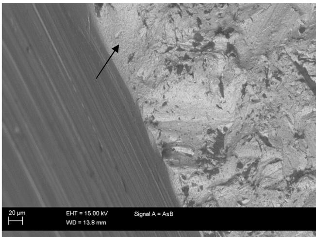
Figure 7. Inner edge of the outer pin of WR6 after the test. Specimen is tilted 45° with respect to the wear surface normal. The arrow points to the marks of fractures close to the edge.
