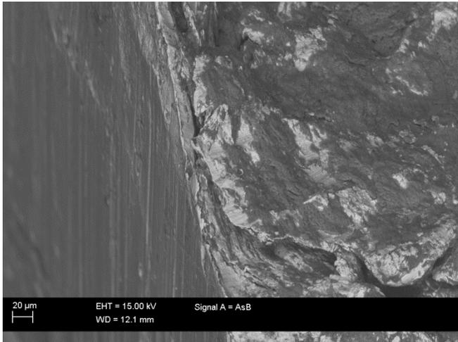
Figure 6. Inner edge of the outer pin of S355 after the test. Specimen is tilted 45° with respect to the wear surface normal. The wear surface is lamellar or flaked close to the edge.
