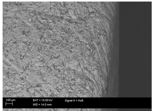
Figure 5. Worn outer edge of the WR6 outer pin after the test. Specimen is tilted 45° with respect to the wear surface normal. Magnification is two times higher than in Figure 4.
