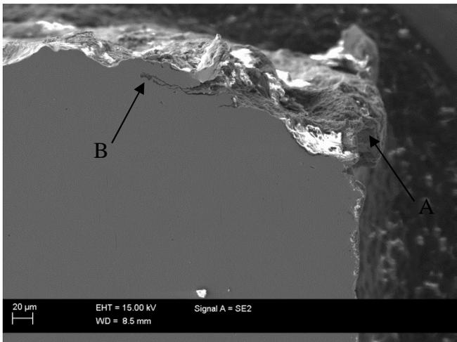
Figure 9. Cross-section of the edge of the S355 inner pin. The edge behind the cross-section protruding from the wear surface (A) and a flake parallel to the wear surface (B) are indicated by the arrows.
