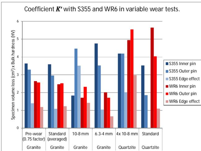
Figure 11. Coefficient  $K'$  for S355 and WR6 in different test steps with granite and quartzite.
