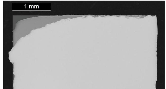
Figure 8. Outer pin cross-sections of both test materials. Dark grey sharp corner is the shape of the pin before the wear test, medium grey is the cross-section of WR6 and light grey the cross-section of S355 after the test.
