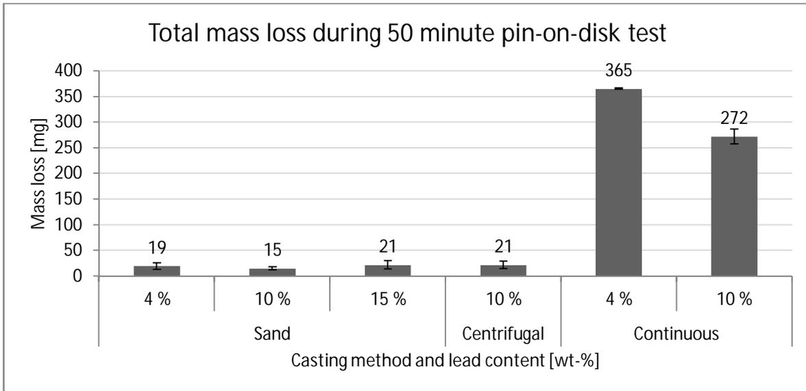
Figure 2. Total mass loss in the pin-on-disk tests.
