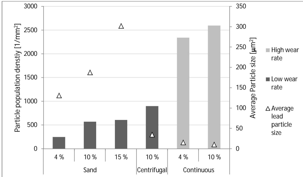
Figure 8. Lead particle population densities of the tested alloys.
