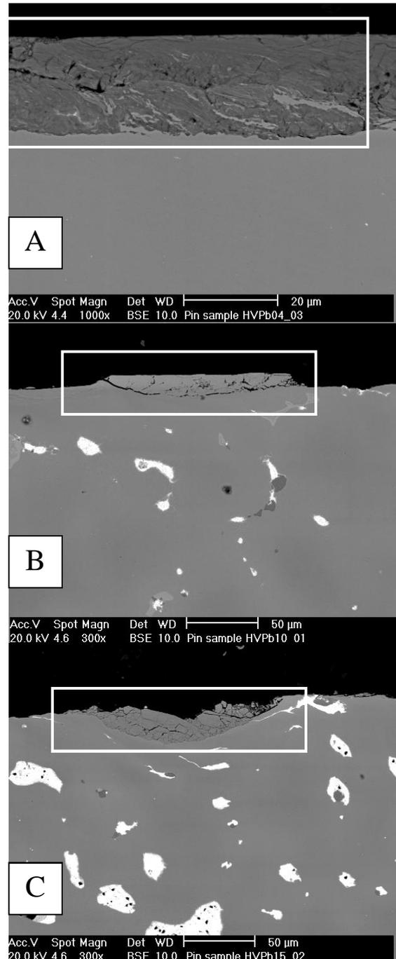
Figure 5. SEM BSE images of distinct layers found on the sand cast samples. A:  $\text{CuSn10Pb4}$  B:  $\text{CuSn10Pb10}$  C:  $\text{CuSn10Pb15}$
