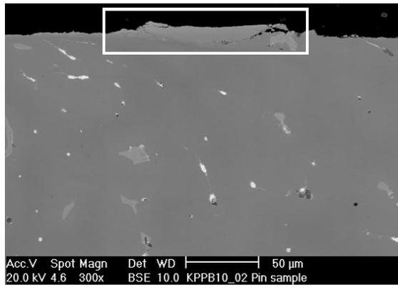
Figure 6. A SEM BSE image of a surface film on the centrifugally cast sample CuSn10Pb10.
