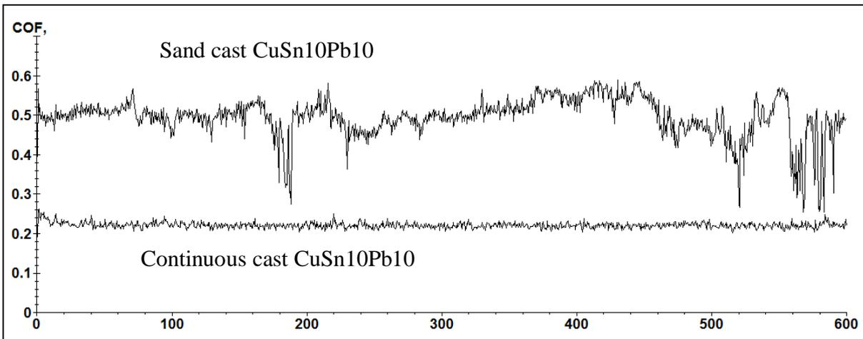
Figure 3. The evolution of the coefficient of friction for sand cast and continuous cast CuSn10Pb10 during a single test run.
