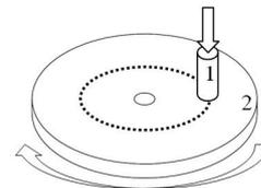
Figure 1. A schematic of the pin-on-disk test setup.
