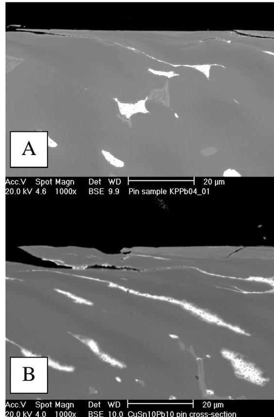
Figure 7. A SEM BSE image of microcracks in the continuous cast samples. A: CuSn10Pb4 B: CuSn10Pb10
