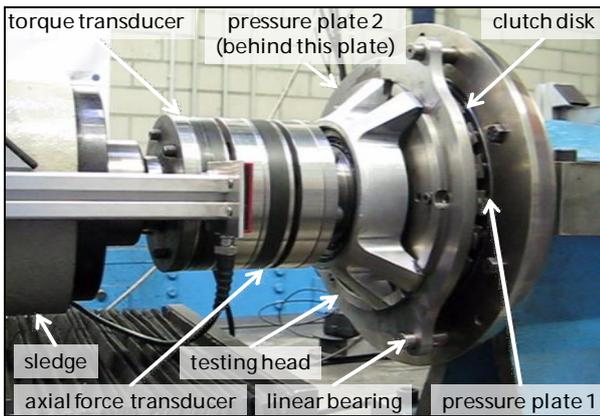
Figure 6. Measurement instrumentation.
