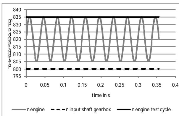
Figure 1. Principle and abstraction of permanent slip.
