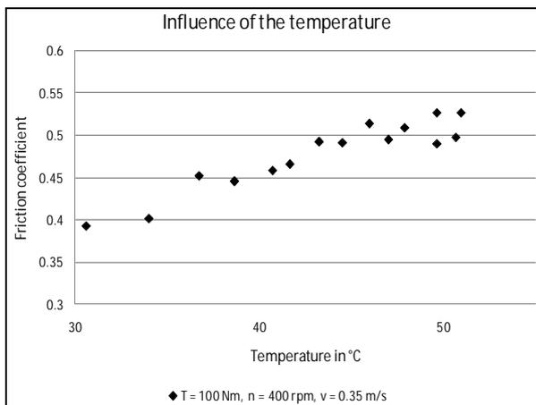
Figure 14. SSiC: Temperature of the pressure plate.
