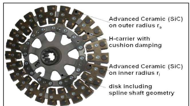
Figure 2. Clutch disk prototype with the advanced ceramic/steel friction pairing SSiC/C45E.
