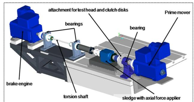
Figure 5. Dry Running Test Bed of IPEK – Setup for the clutch disk prototype
