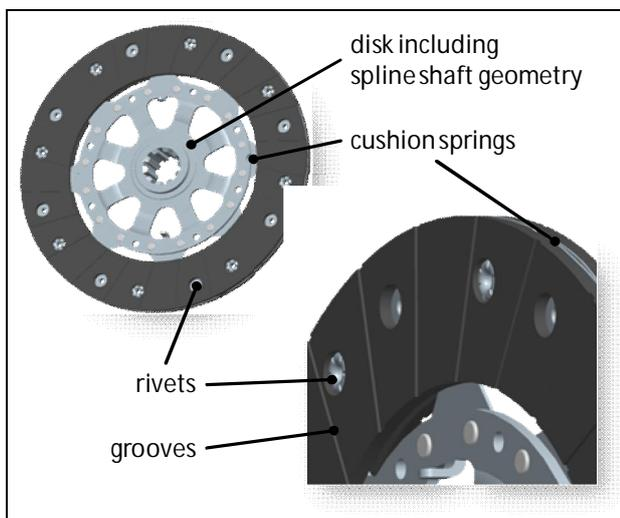
Figure 4. Reference clutch disk with an organic facing.
