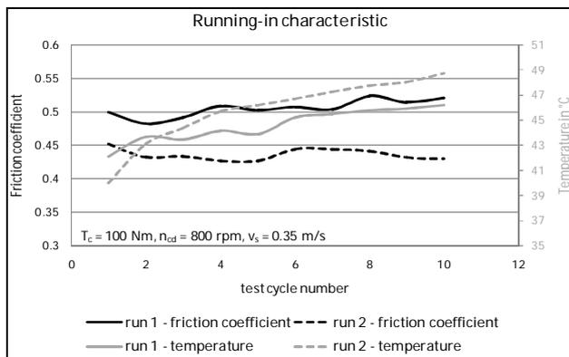
Figure 10. SSiC: Running-in characteristic.
