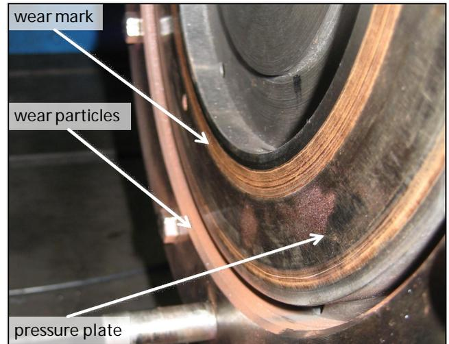
Figure 18. Ceramic pressure plates after testing.
