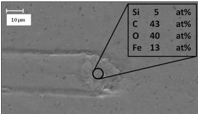
Figure 17. SSiC: EDX analysis of a hotspot.
