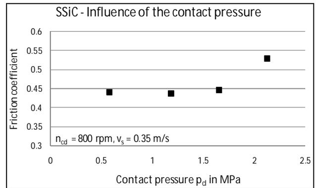
Figure 11. SSiC: Contact pressure.
