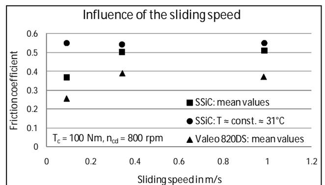
Figure 13. SSiC, Valeo 820DS: Sliding speed
