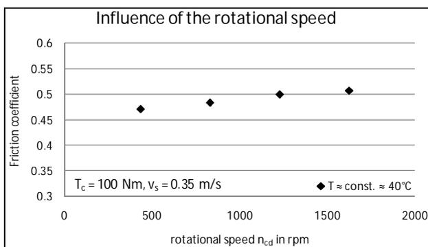
Figure 15. SSiC: Rotational speed.
