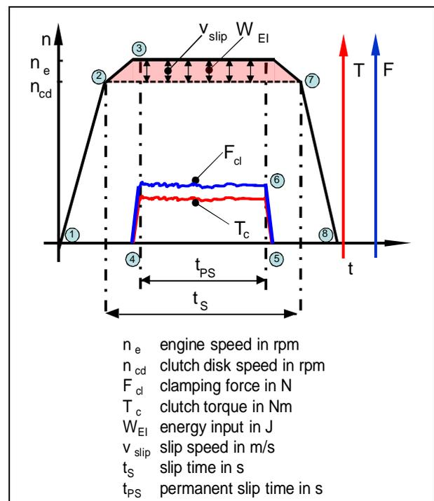
Figure 7. Test procedure for permanent slip cycles.
