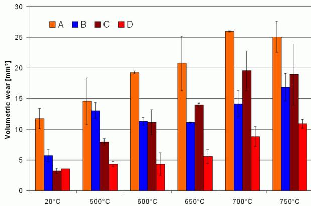
Figure 6. CIAT wear rates of the tested alloys at different testing temperatures.
