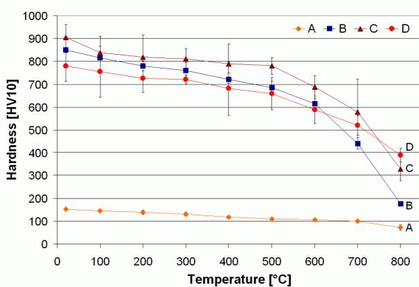
Figure 5. Hot hardness HV10 determined at temperatures from RT up to 800°C.
