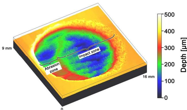
Figure 4. Surface topography obtained in the confocal microscope and used for volumetric wear calculation.
