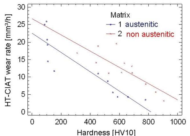
Figure 7. HT-CIAT wear rates correlated to hot hardness
