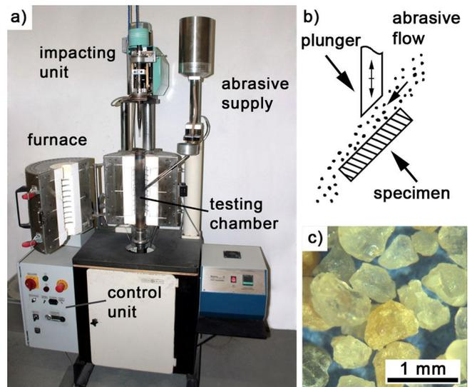
Figure 3. (a) View of the High Temperature Cyclic Impact Abrasion Tester (HT-CIAT), (b) testing principle (45° impact angle with abrasives tested) and (c) abrasive.
