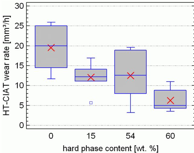
Figure 8. Box and whisker plot of HT-CIAT wear rates correlated to hard phase content.
