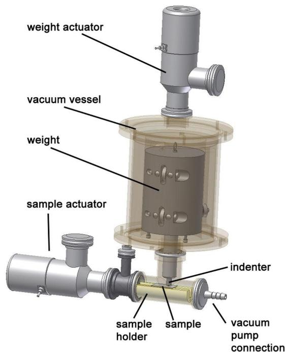
Figure 2. Hot hardness measurement system developed by AC<sup>2</sup>T.
