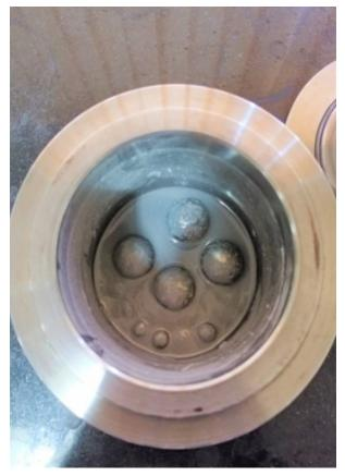
Figure 2. Ball mill powder in toluene medium
