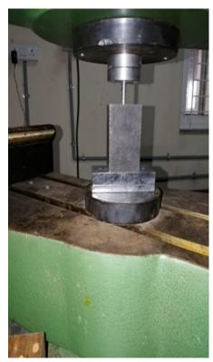
Figure 3. Uni-axial compaction under UTM
