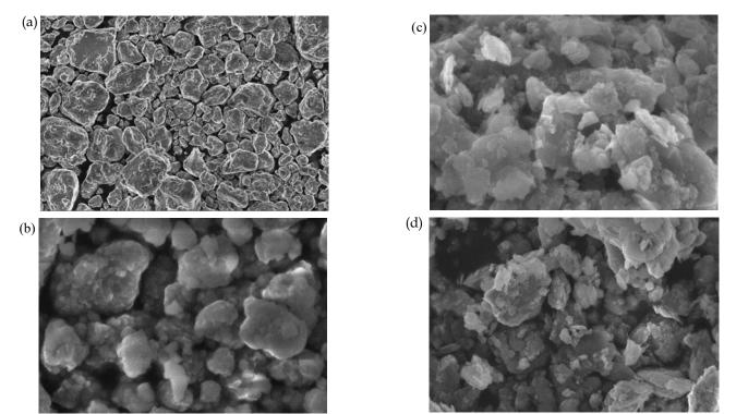
**Figure 6 (a-d).** SEM micrographs of sintered composites (a) Al 7075, (b) Al 7075 -5% SiC, (c) Al 7075-5 SiC-5% Gr, (d) Al 075-5 SiC-10% Gr
