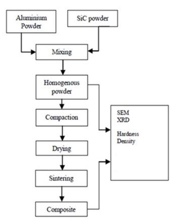
Figure 1. Powder metallurgy process chart
