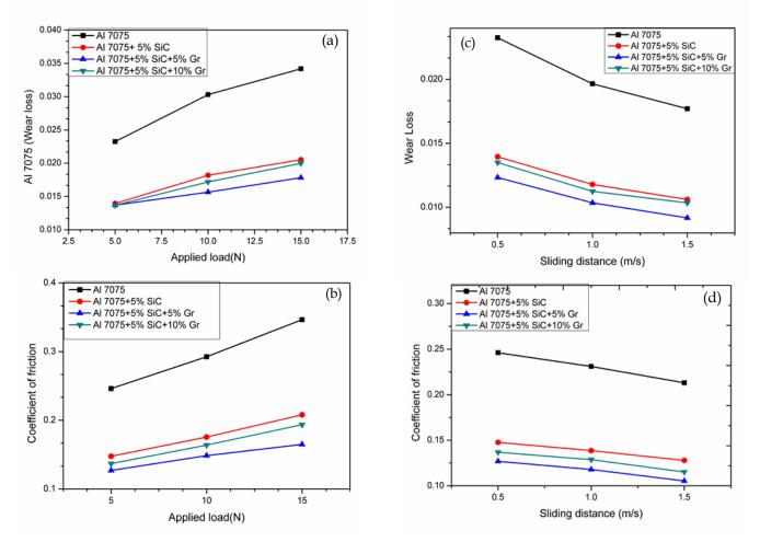
**Figure 9(a-d):** (a)wear loss Vs applied load, (b): coefficient of friction Vs Applied load, (c) waer loss Vs sliding distance, (d) coefficient of friction Vs sliding distance.
