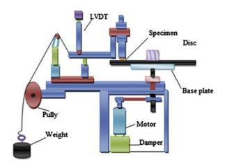
**Figure 5.** Schematic view of the pin-on-disc apparatus used in the study
