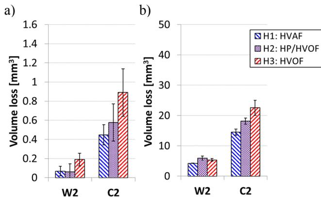
Figure 1. Volume loss of the coatings after a) slurry erosion test with fine quartz and b) with coarse quartz.
