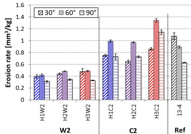
Figure 2. Erosion rate of WC-10Co4Cr coatings (W2), Cr<sub>3</sub>C<sub>2</sub>-25NiCr coatings (C2) and reference samples after dry erosion tests at 30°, 60° and 90° impact angles
