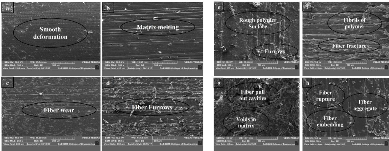
**Figure 3.** The SEM images of the worn surfaces of GC hybrid composites under the influence of sliding load: a) Blend (PA66/PTFE)(75 N), b) Blend (PA66/PTFE)(150 N), c) Blend(PA66/PTFE)/SGF (75 N), d) Blend(PA66/PTFE)/SGF (150 N), e) Blend(PA66/PTFE)/SCF (75 N), f) Blend(PA66/PTFE)/SCF (150 N), g) GC hybrid composites (75 N) and h) GC hybrid composites (150 N)
