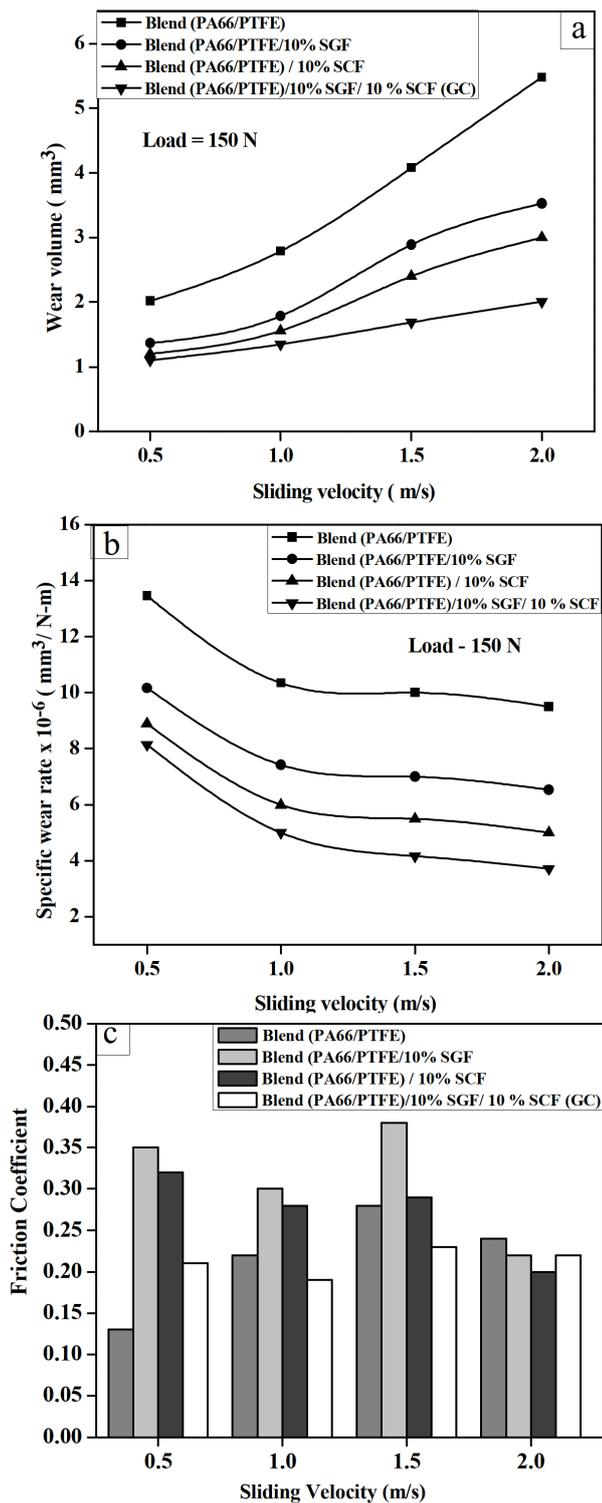
**Figure 4.** Tribological response of fiber filled and GC hybrid composites under varying experimental velocity: a) Volume loss, b) Wear rate and c) Frictional constant
