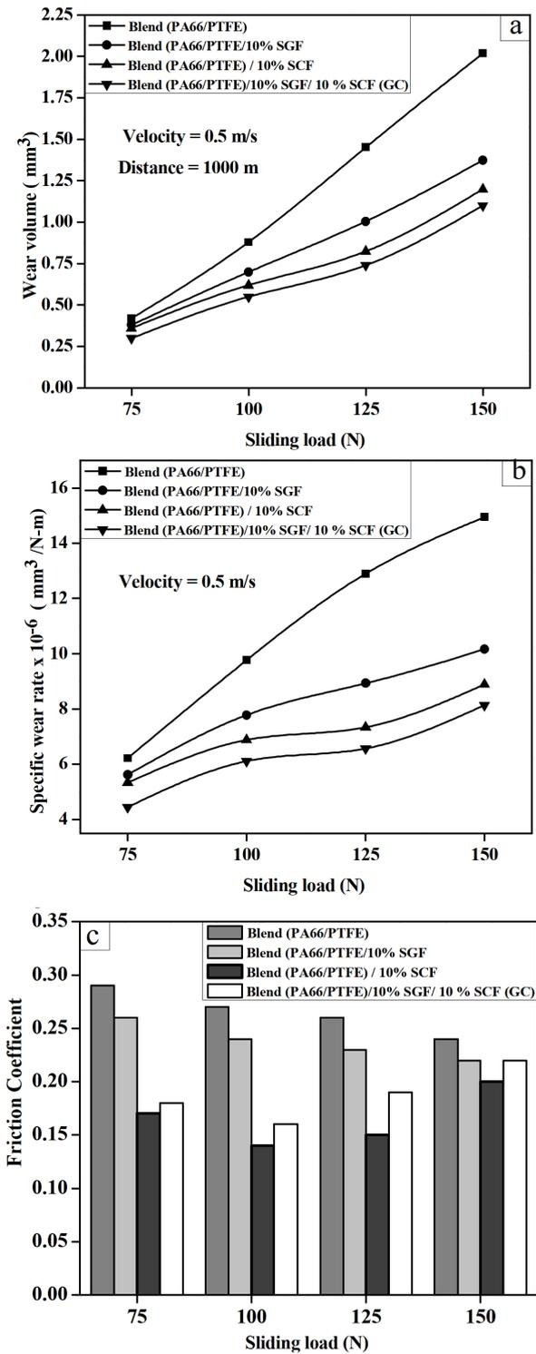
**Figure 2.** Tribological response of GC hybrid composites under varying experimental load: a) Volume loss, b) Wear rate and c) Frictional constant
