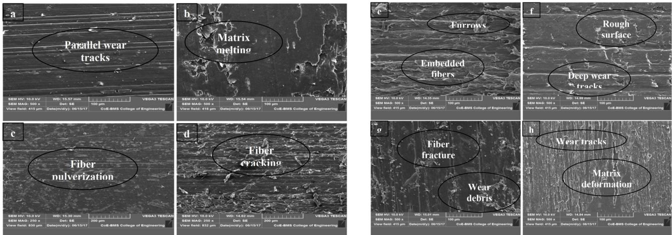
**Fig 5.** The SEM images of the worn surfaces of fiber filled and GC hybrid composites under the influence of sliding velocity: a) Blend (PA66/PTFE)(0.5 m/s), b) Blend (PA66/PTFE)(1 m/s), c) Blend (PA66/PTFE)/SGF (0.5 m/s), d) Blend (PA66/PTFE)/SGF (2m/s), e) Blend (PA66/PTFE)/SCF (0.5 m/s), f) Blend (PA66/PTFE)/SCF (2 m/s), g) GC hybrid composites (0.5 m/s) and h) GC hybrid composites (2 m/s)
