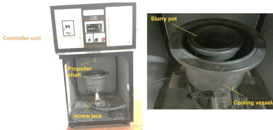
FIGURE 3. Photograph of the erosion wear pot tester.
