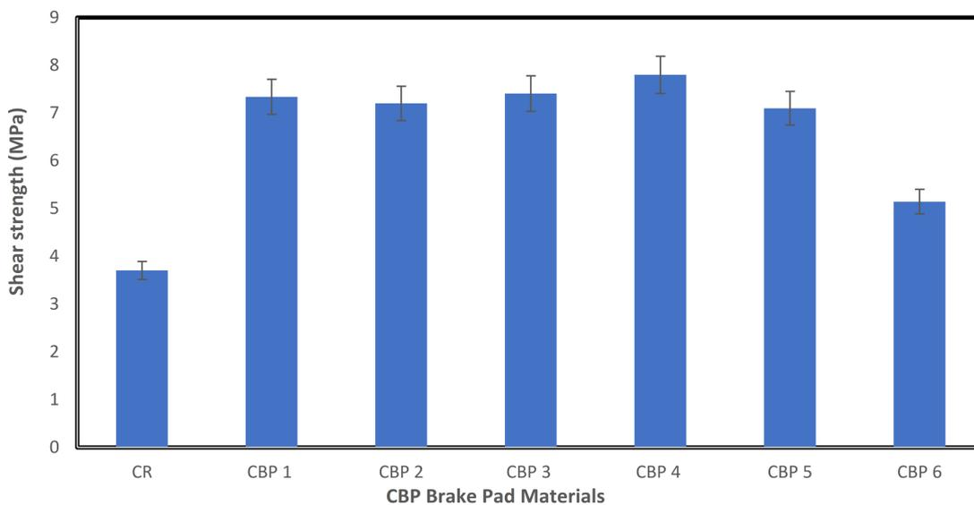
**Figure 3:** Shear strength of carbon-based and commercial friction materials.
