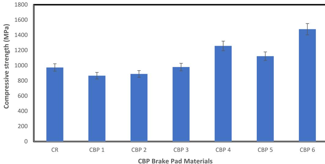
**Figure 1:** Compressive strength of carbon-based and commercial friction materials.
