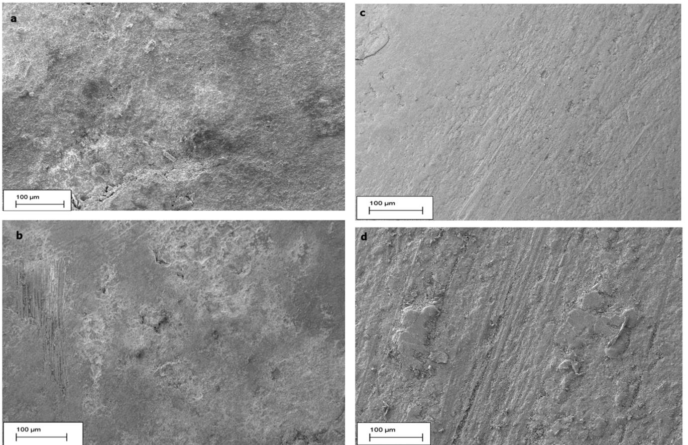
**Figure 7:** SEM micrographs showing worn surfaces of; (a) C.R. before soaked in oil (b) C.R. after soaked in oil (c) CBP before
