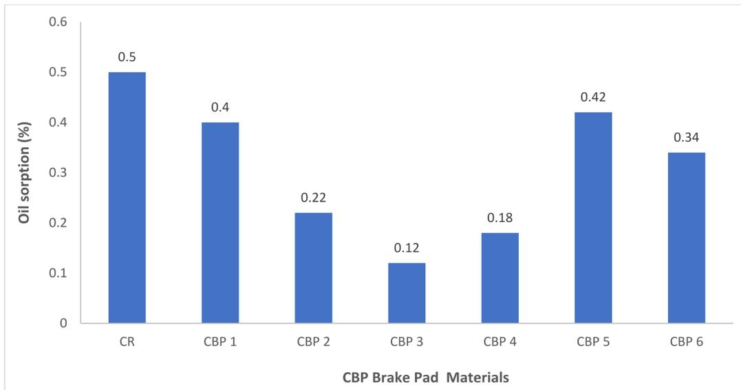
**Figure 6:** Histogram showing the oil absorption rate of carbon-based and commercial friction materials.
