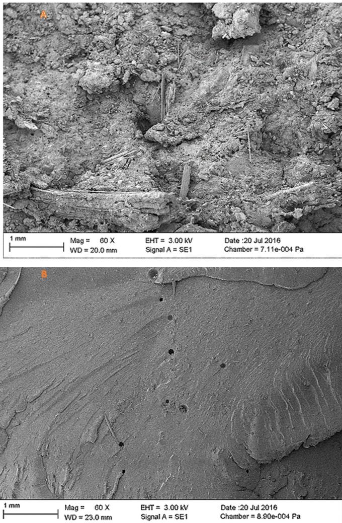
**Figure 4:** SEM micrograph showing shear fracture surface of (A) commercial brake pad material and (B) carbon-based brake pad material
