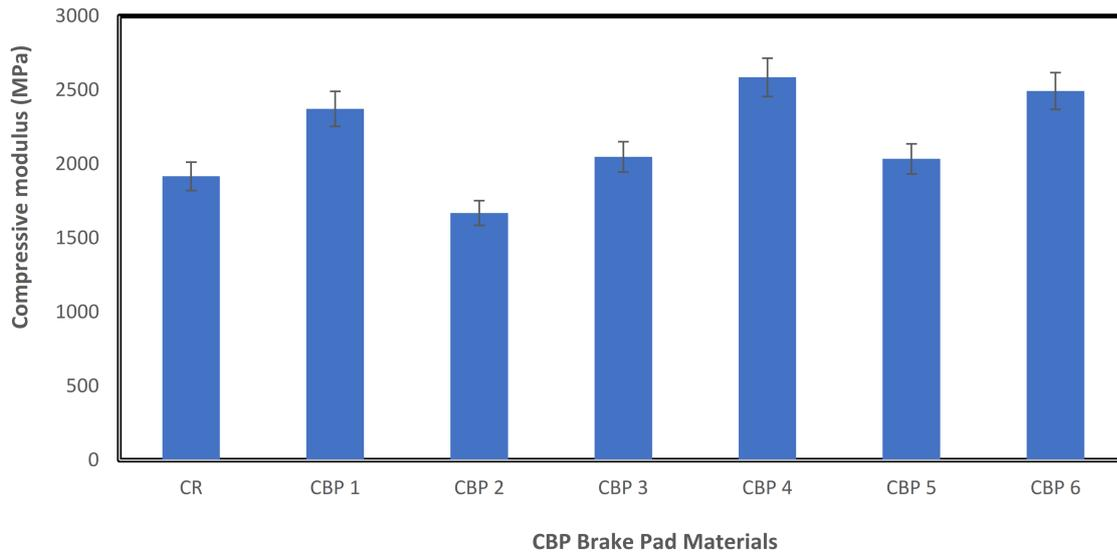
**Figure 2:** Compressive stiffness of carbon-based and commercial friction materials.
