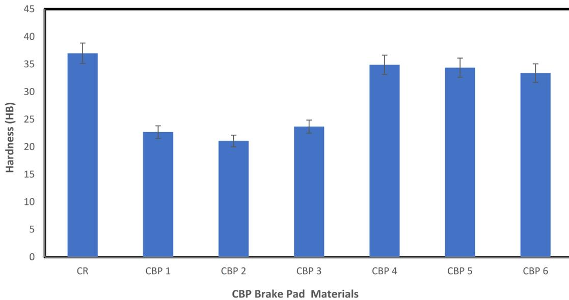
**Figure 5:** Hardness properties of carbon-based and commercial friction materials.
