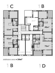
FIGURE 4 Case 1, the original building plan on the left and the proposed modified building plan on the right. The grey colour highlight the focus apartments in this study. The staircases are highlighted with hatched pattern. The adaptation potential of cases is separately evaluated in Tables 2 and 4.
