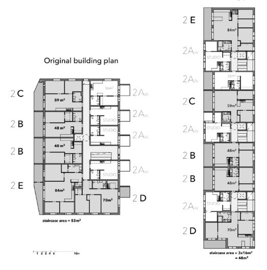
FIGURE 5 Case 2, the original building plan on the left and the proposed modified building plan on the right. The grey colour highlight the focus apartments in this study. The staircases are highlighted with hatched pattern. The adaptation potential of cases is separately evaluated in Tables 3 and 5.
