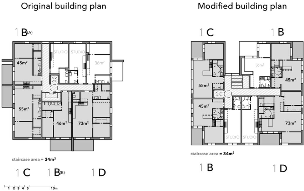
**FIGURE 4** Case 1, the original building plan on the left and the proposed modified building plan on the right. The grey colour highlight the focus apartments in this study. The staircases are highlighted with hatched pattern. The adaptability potential of cases is separately evaluated in Tables 2 and 4.
