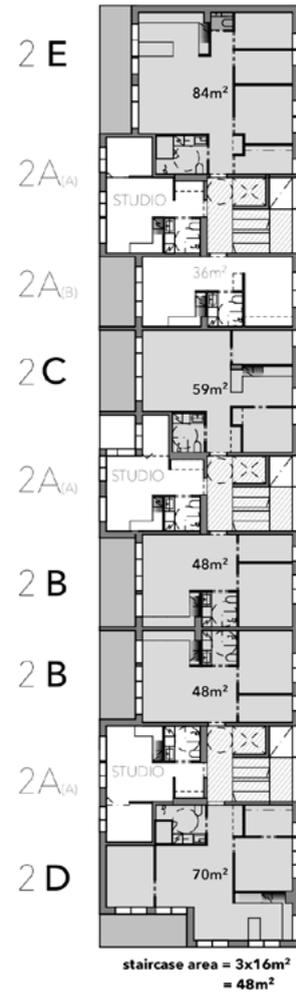
**FIGURE 5** Case 2, the original building plan on the left and the proposed modified building plan on the right. The grey colour highlight the focus apartments in this study. The staircases are highlighted with hatched pattern. The adaptation potential of cases is separately evaluated in Tables 3 and 5.
