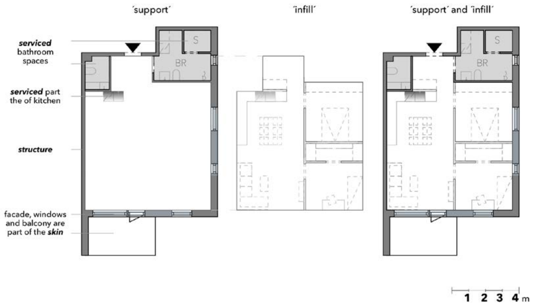
FIGURE 1 Illustration of the difference between the apartment 'support' (on the left) and 'infill' (in the middle), as used in this study. The illustration on the right presents 'support' and 'infill' together. The apartment 'support' i.e. community-controlled and slower changing building aspects, as used in this study, is highlighted in darker grey. The apartment 'infill', as used in this study, can be adjusted more easily by dwellers, and is highlighted in lighter grey. Storage cabinets and replaceable furniture are highlighted in a light grey dashed line. The arrow indicates the apartment entrance.
